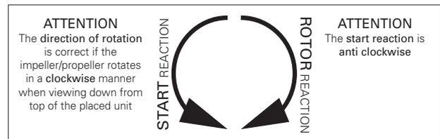
For large pumps, the direction of rotation can also be recognized by looking through the pressure socket into the pump chamber. Here the impeller can be seen and after briefly switching it on, during the outflow from the impeller, the direction of rotation can be controlled.
