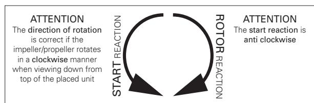
For large pumps, the direction of rotation can also be seen by looking into the pump chamber through the pressure port. The impeller can be seen here and can be switched on after a short while, when the impeller runs out, check the direction of rotation
