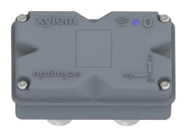
By periodically monitoring vibration, temperature and magnetic flux, optimyze is able to identify potential problems with your equipment before they occur. Health information is collected, stored and analyzed in the optimyze sensor before being wirelessly transmitted to your iOS or Android smart device via Bluetooth. The optimyze mobile application provides an easy interface to understand the health of your assets, create maintenance reminders and generate detailed reports.
