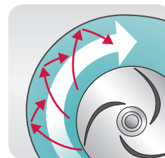
Standard impeller slams solids into the volute.
